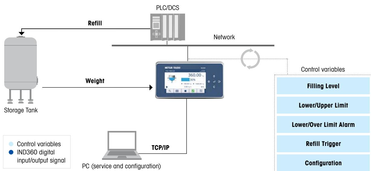
PLC controls the refill valve based on IND360 refill signal and other control information, the IND360 monitors the filling level and provides visualization on HMI. Cyclic and acyclic access to application status information and read/write of configuration using PLC interface, display or web interface. Redundant ring topology for PROFINET and EtherNet/IP is supported.
