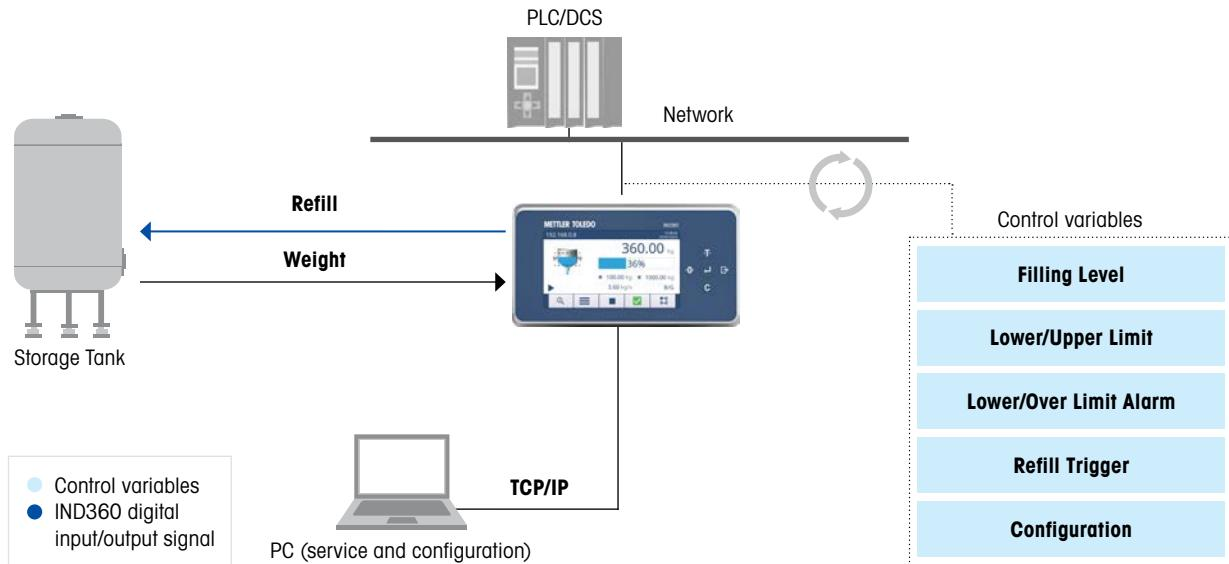
IND360 controls the refill valve while providing visualization on HMI. Cyclic and acyclic access to application status information and read/write of configuration using PLC interface, display or web interface. Redundant ring topology for PROFINET and EtherNet/IP is supported.
